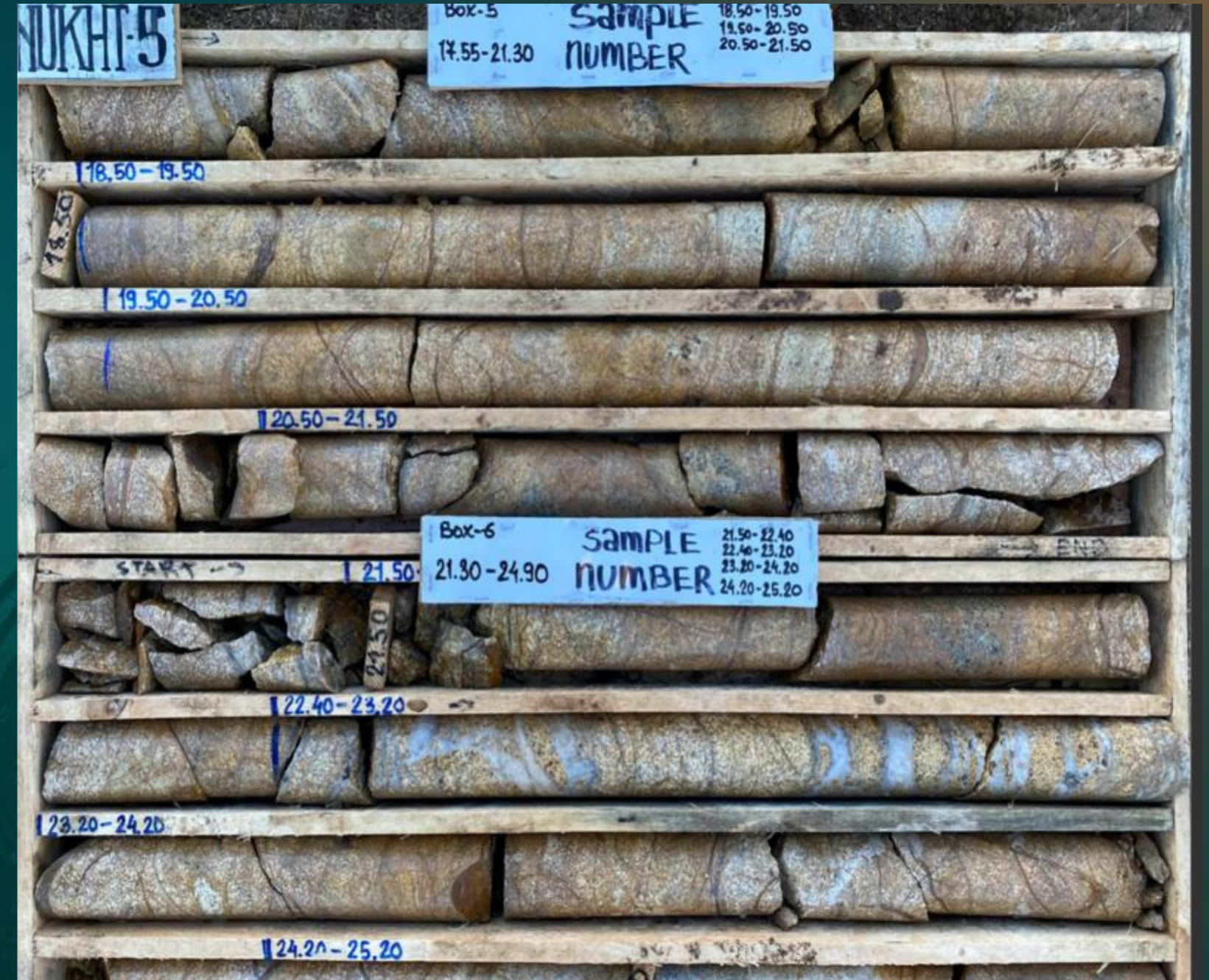
Nukht site near Gyalalzakh area quartz veins with 10 g/t gold mineralization
