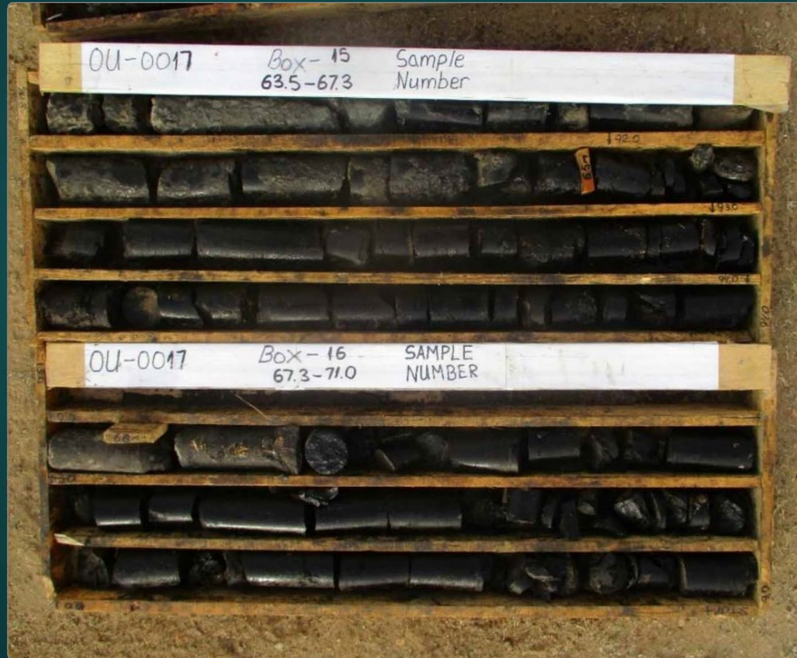
Olongiin Ukhaa brown coal deposit's OU-0017 borehole drill core at 63.5-71.0 m
