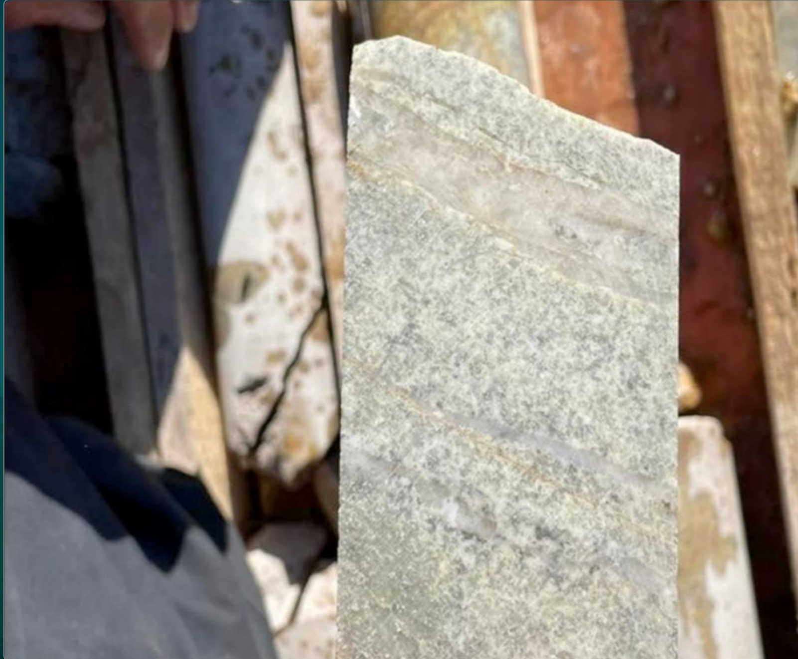
NUKTH-01 borehole at 31.50-39.35 m, Au-0.9 g / t grade quartz granite, 2-3% pyrite mineralization, strong quartz-sericitized granodiorite
